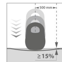
This factor measures the spread of deformation of the surface finish that might occur as a result of dynamic impact. Acceptable deformation is within 500mm from point of impact, 15% of total deformation at the point of impact. This indicator is standardized to ensure that any impact that an athlete has on the flooring surface does not distort ball bounce or trajectory.
