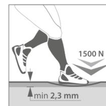
Deformation of a flooring surface following dynamic impact of 1500 N. This indicator is measured in conjunction with shock absorption, and its optimal range is 2.3mm to 5 mm.
