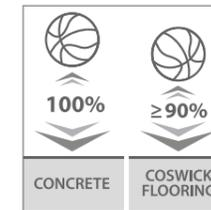
This indicator is required for games and activities that involve a bouncing ball. The test compares the bounce ball measure of a fully inflated basketball to the bounce from a concrete surface. The resulting indicator must be at least 90% of the bounce from concrete.
