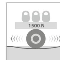
Operational factor that indicates the suitability of the flooring surface for enduring heavy carts with rubber wheels that are frequently used to move various sports equipment. The tests are carried out with a load of 1500 N (153 kg).
