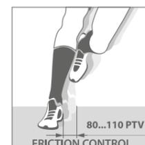
This factor measures resistance to sliding upon impact of clean athletic shoes on a dry flooring surface. The test uses a special pendulum device, and requirement measurement needs to fall within 80 and 110 range. A lower result indicates that the floor is too slippery, while a higher suggests that athletes' will "stick" to the floor, limiting their range of movement. Surface friction impacts athlete's ability to move along a complex trajectory.
