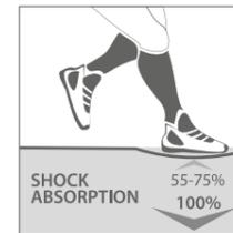
Shown as a percentage, shock absorption represents the extent, to which a sports floor covering is able to soften an athlete's landing, as compared to an inflexible surface (e.g., concrete slab). The best types of sports floors are required reduce the impact by 55 to 75%. This is the optimal range that ensures athletes' comfort without compromising speed or performance.
